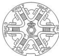
7-way trailer plug - car end-rear view
