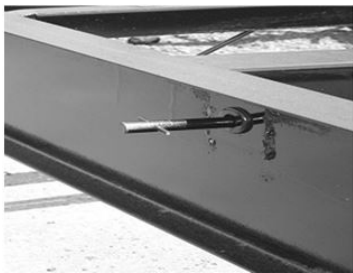
Fig. 1-Through Frame Crank Extension w/pin
