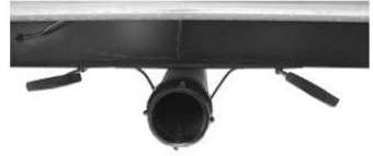
Black/Grey tank drain & valves
